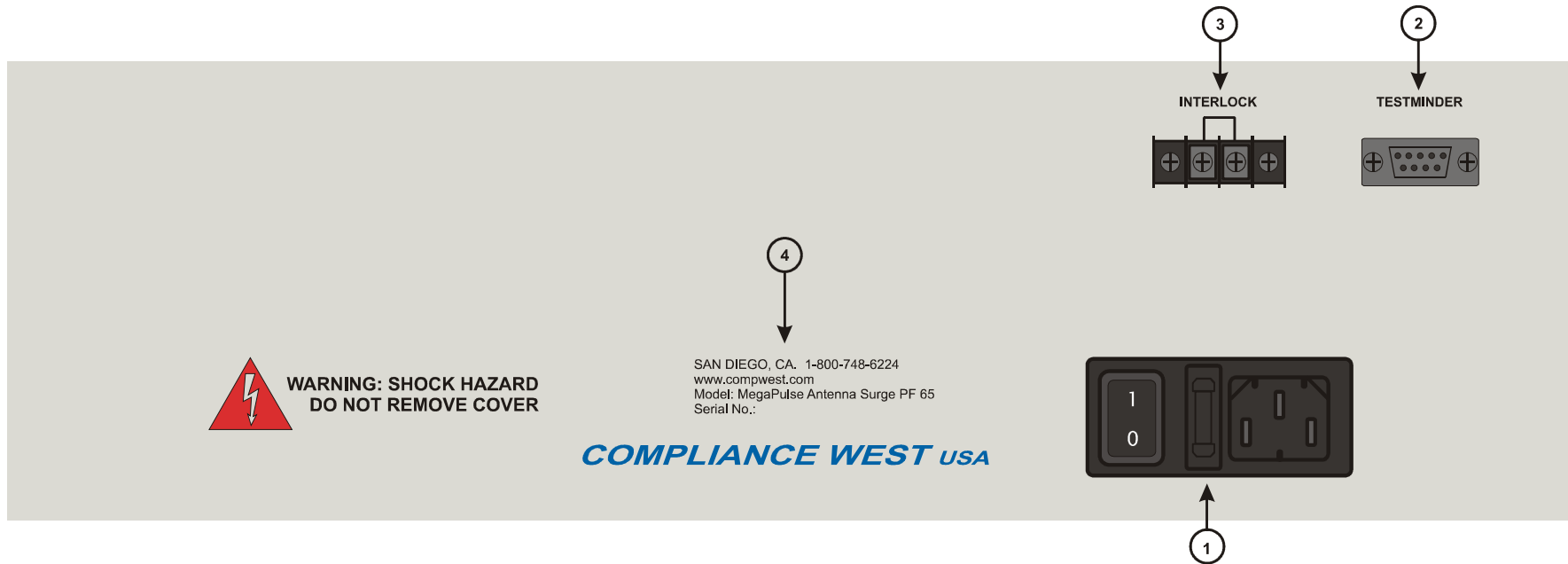
Figure 3. Controls, Indicators, Connectors – MegaPulse Antenna Surge PF Rear Panel.
